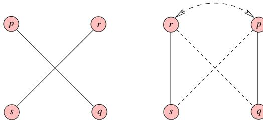
**Fig. 8.** The  $\text{flip}(e_1, e_2)$  operation.
